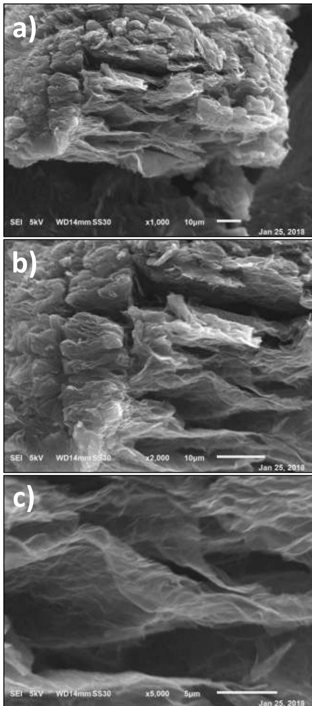
Figure 1. SEM micrographs of commercial graphene particles Avanzare powder a) 1000x, b) 2000x and c) 5000x magnification.
