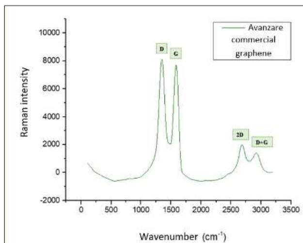
Figure 3. Raman spectrum of commercial graphene Avanzare.
