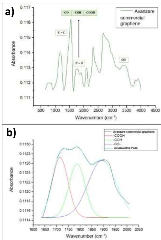
Figure 2. FTIR spectra of commercial graphene Avanzare a) total range and b) deconvolution in the range of oxygenated groups with the carbonyl group (C = O).
