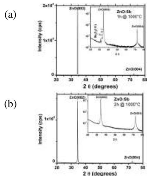
**Figure 1.** XRD patterns of ZnO samples (a) after 1 h of diffusion (b) after 2 h of diffusion.
