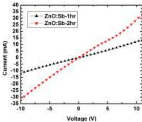
**Figure 4.** I-V Curves for ZnO samples with different periods of diffusion.
