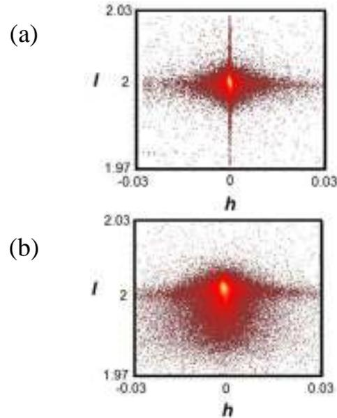
**Figure 3.** HRXRD reciprocal space maps of ZnO samples (a) before the diffusion (b) after 2 h of diffusion.
