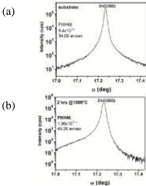
**Figure 2.** HRXRD rocking curves of ZnO samples (a) before the diffusion (b) after 2 h of diffusion.
